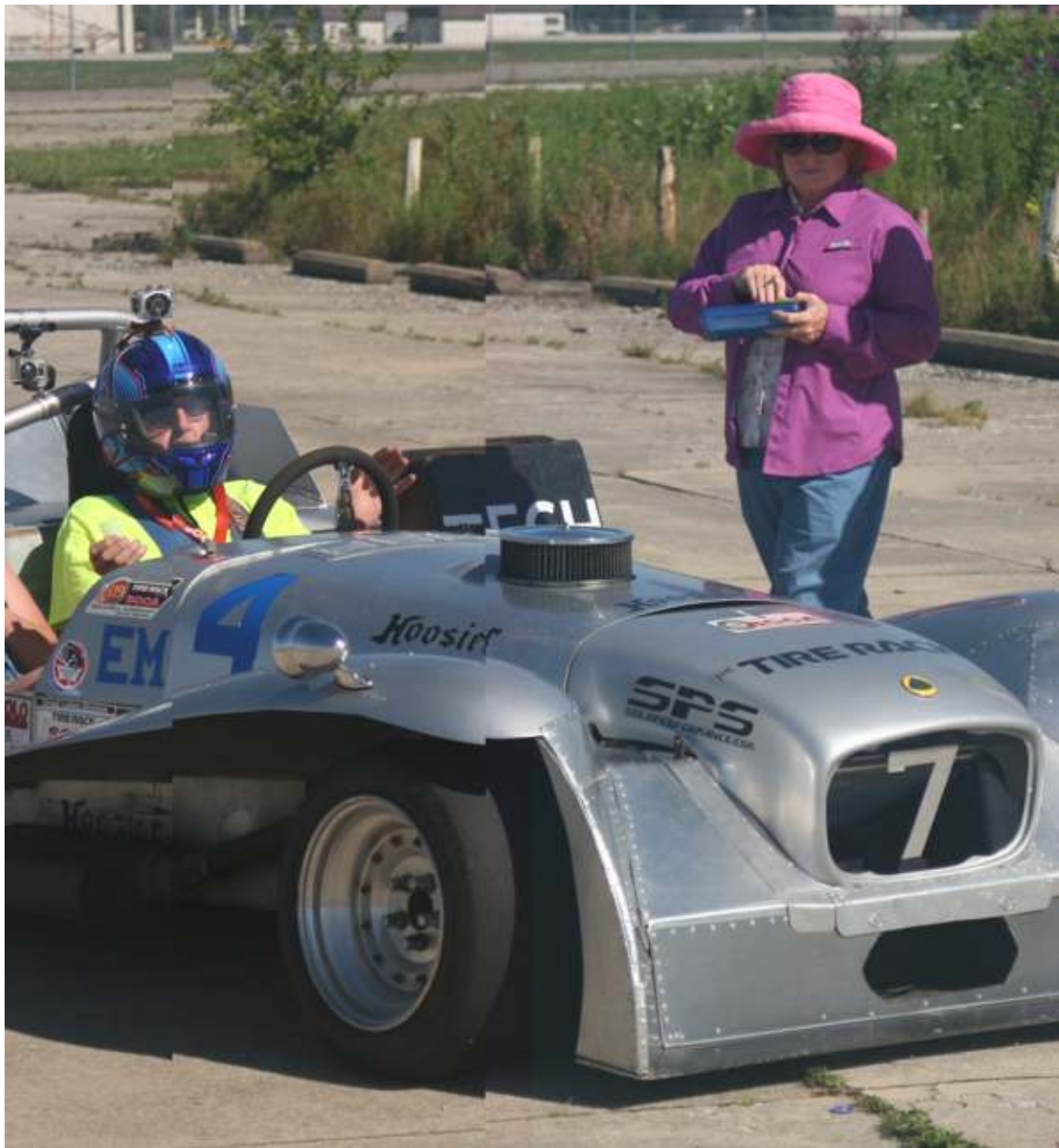
Lee Miller's version of an air dam...more like a air plow. All them rivets gives it kinda WW2 aircraft look, dontcha think?
